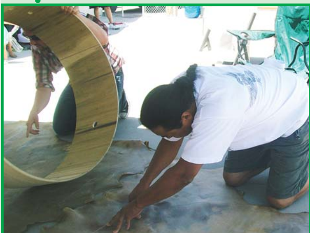
Step 5: Cut skin with sharp blade or utility knife.
